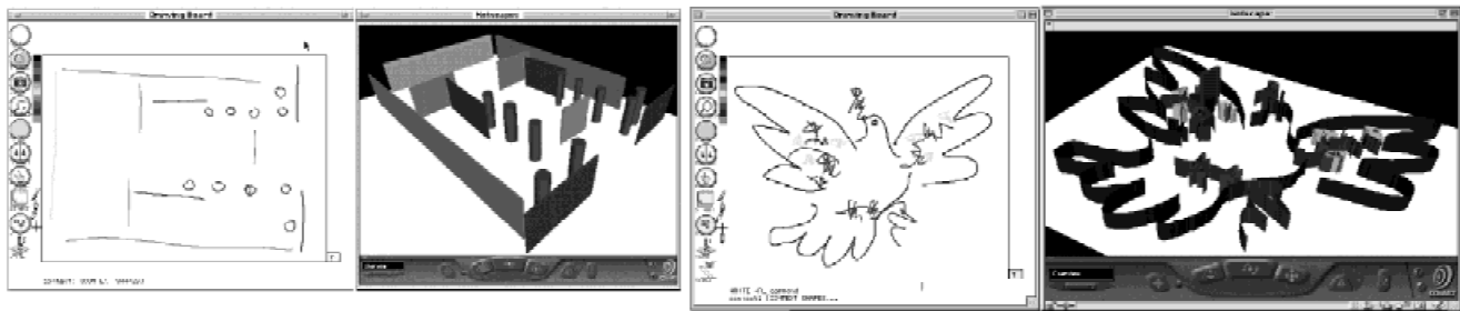
Fig. 32. Sketch-VR extrudes lines, circles, and curve shapes as wall lines to make floor plan partitions.
