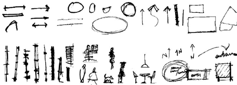
Fig. 8. Top: primitives (drawing elements) used in drawing included arrows, lines, hatches and simple geometric shapes. Bottom: symbols (architectural objects) such as walls, windows, and stairs are formed by combination of primitives.
